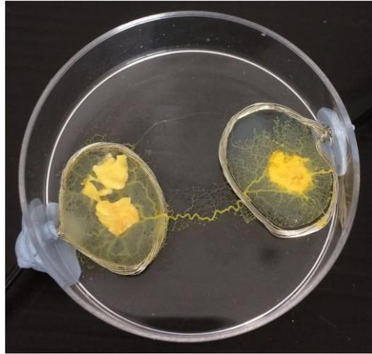
Figure 5: A photograph of the control samples' experimental setup. Shown is two electrodes comprised of a circle of wire filled with non-nutrient agar, linked by a protoplasmic tube.
