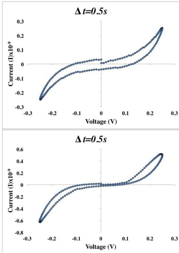
Figure 9: Two I-V graphs recorded under the lowest voltage range (250mV) and quickest time step ( $\Delta t=0.5$ ). We recorded the top graph using a 10mm receptacle, and the bottom graph using a 2.5mm receptacle. The 2.5mm receptacle's profile was closer to touching at origin under these test conditions.
