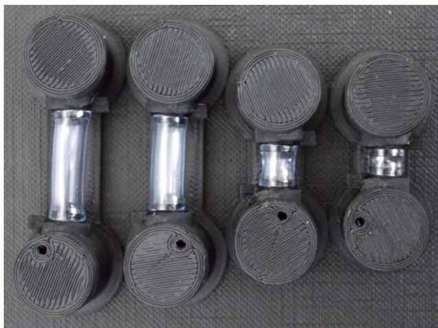
Figure 4: A photograph of our receptacles set up with different tube lengths to investigate the effect on memristance. Shown are connecting tube lengths of 2.5mm, 5mm, 15mm and 20mm.
