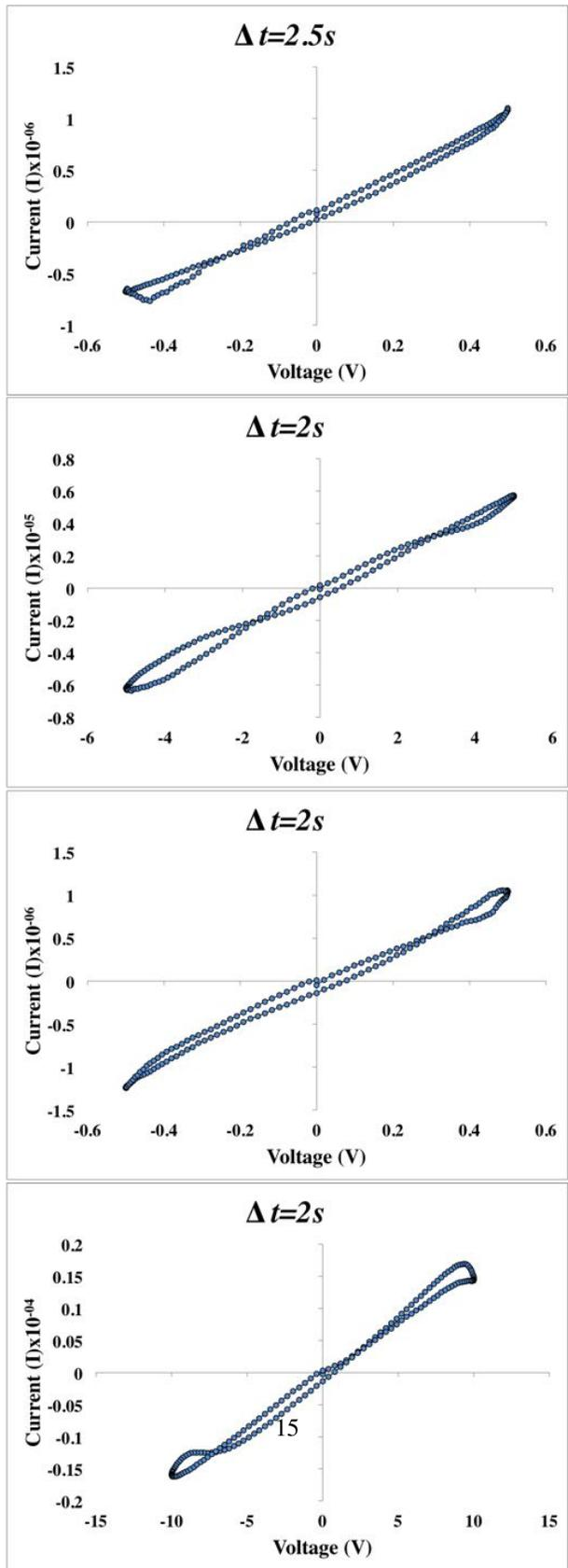
Figure 10: Four pinched I-V curves measured on the our control samples. Results with these samples presented a high degree of variation sample-to-sample. Furthermore, in several cases, the memristive curves had several pinch points
