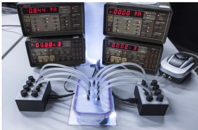
Figure 13: We have begun fabricating plug and play USB ‘PhyBoxes’ that the receptacles presented in this paper clip into. Our PhyBoxes encompass four *P. polycephalum*-based memristors, which are each independently addressable via a USB connection. Depicted in this Figure are two PhyBoxes and a custom-made humidity pump.
