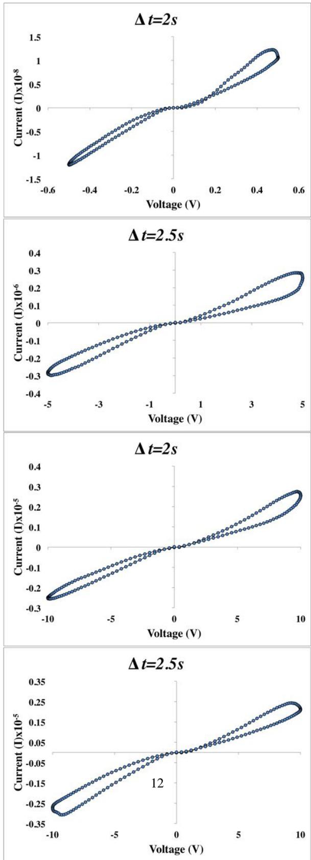
Figure 8: Four examples of pinched I-V curves measured on the 10mm receptacle samples. Notice how each curve is morphologically similar in regards to location of pinch points and lobe sizes.
