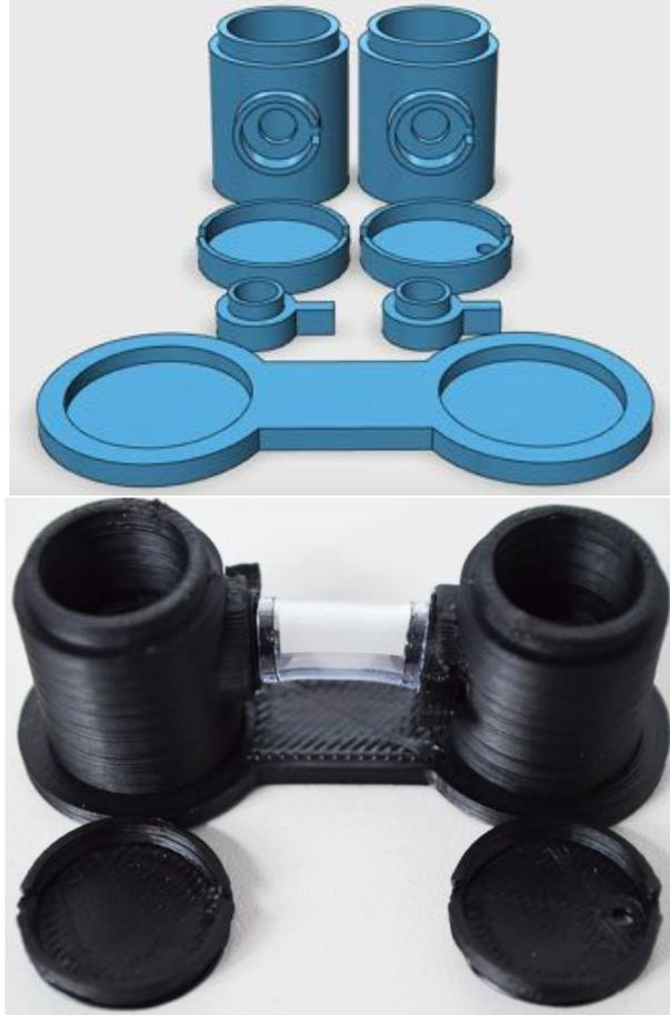
Figure 3: A screenshot (top) and photograph (bottom) of our receptacle. Shown is two identical growth chambers, two lids (one with and one without an air hole), two conductive electrode collars and a 10mm base.
