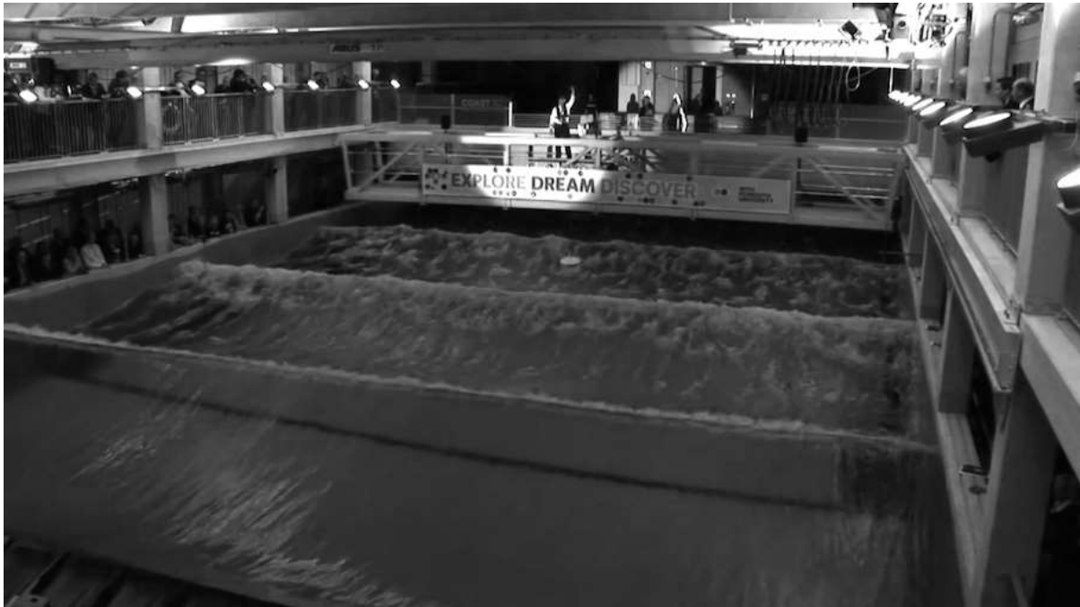
Fig. 3. Over-driven Sine wave during demonstration; the demonstrator can be seen in spotlight on the bridge-like gantry, and the buoy in the water below .
