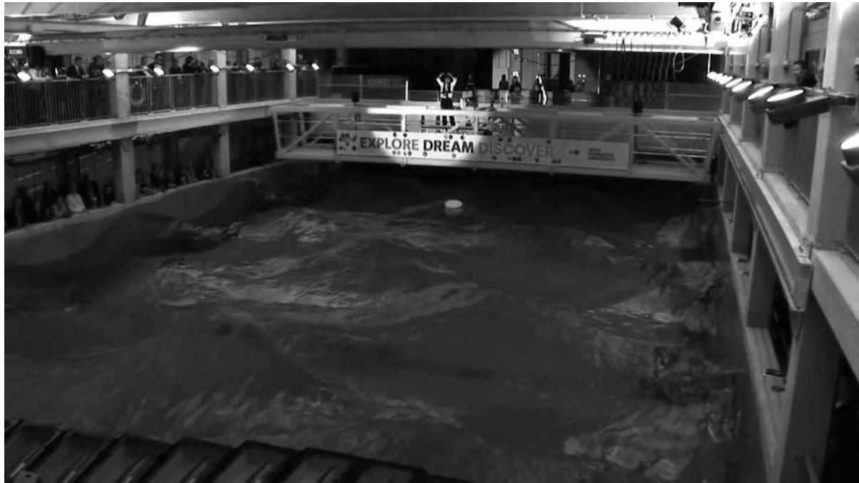
Fig. 4. Quilt wave (small) during demonstration; the wave paddles in motion can be seen in lower left of the image.
