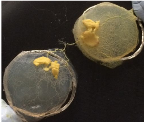
Fig. 4. A P. polycephalum component grown between two electrodes comprised of a circle (approximately 2cm in diameter) of tinned copper wire (16 stands at 0.2mm) filled with a 2-percent non-nutrient agar.
