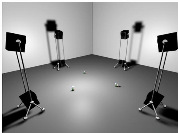
**Figure 1.** *Auditory Sphere. 8 active speakers angled to provide versatile software controlled diffusion. Diffusion and synthesis generated from environment/interaction data collected by each Orb. Software developed in MAX/MSP running on G4 Apple laptop with M-Audio 410 Firewire mobile multi - channel interface, custom built 'composer - listener' objects (Orb3 interfaces)*
