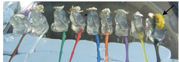
Fig. 2 Photo of an example setup. The reference electrode is on the right side. The other 8 electrodes are measurement electrodes. They are covered with blobs of non-nutrient agar and oat flakes placed on top of each. At the beginning, a piece of plasmodium is placed on top of agar blob covering the reference electrode only (indicated by the arrow).
